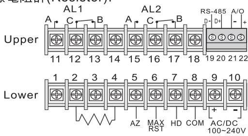
● 2線電阻計(Resistor):
